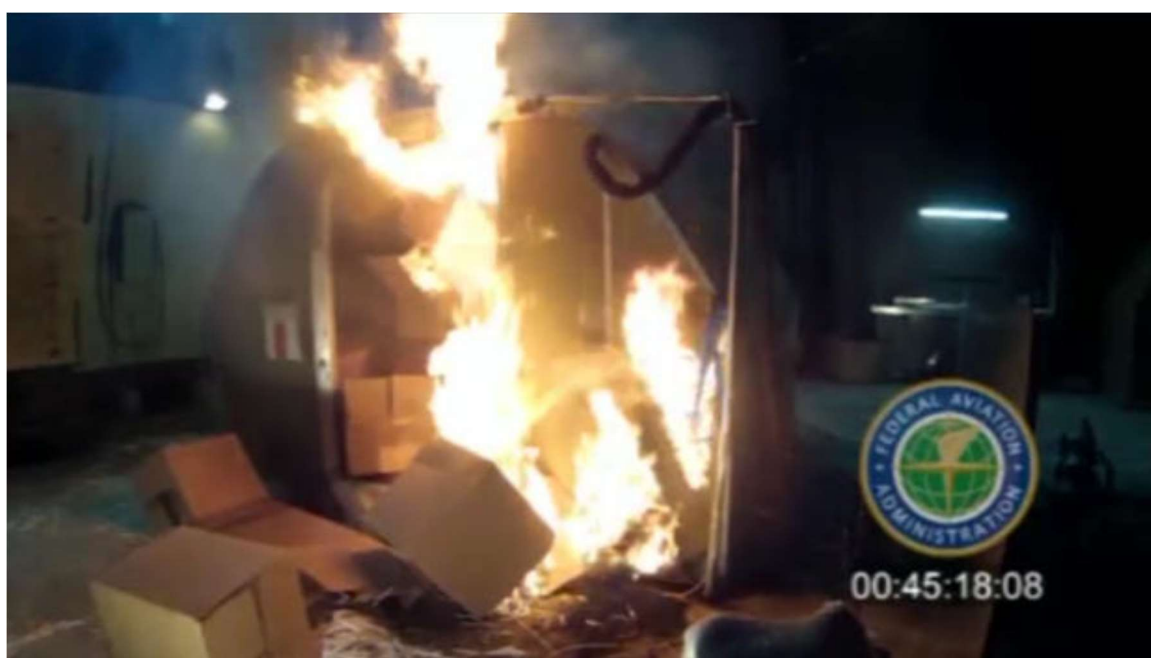
Figure 1.1: Cargo Container Explosion Caused by Lithium Battery Vent Gases
