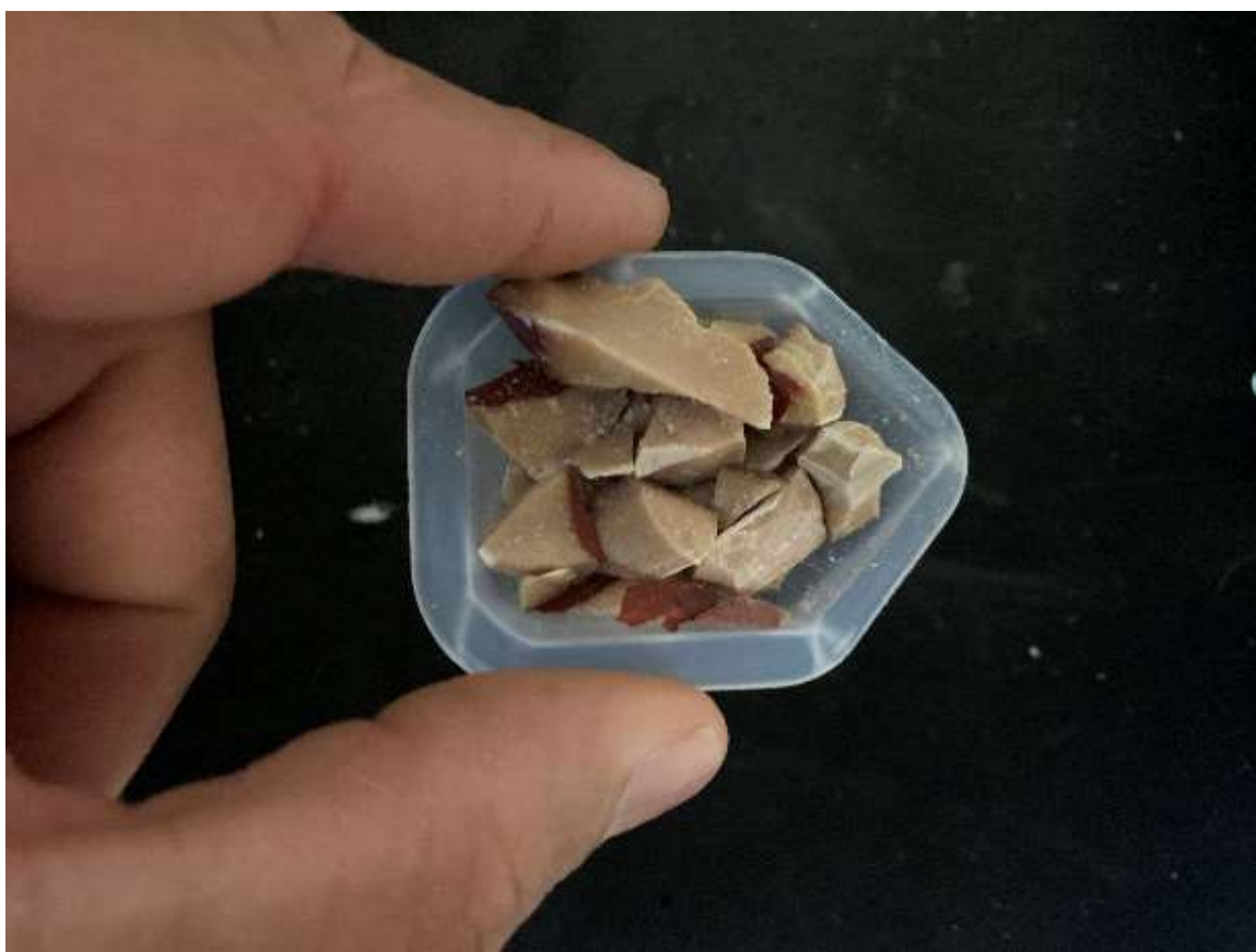
Figure 2.12 Pre-Weighed Solid Aerosol Chunks Prior to Insertion into the Pressure Vessel
