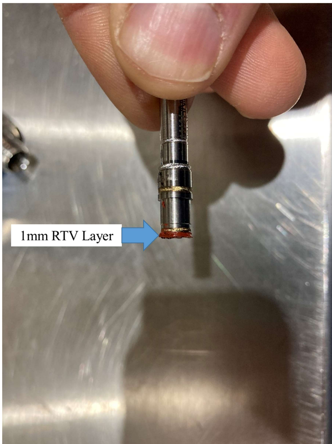
Figure 2.2: 1mm RTV Layer on Piezo Electric Pressure Sensor
