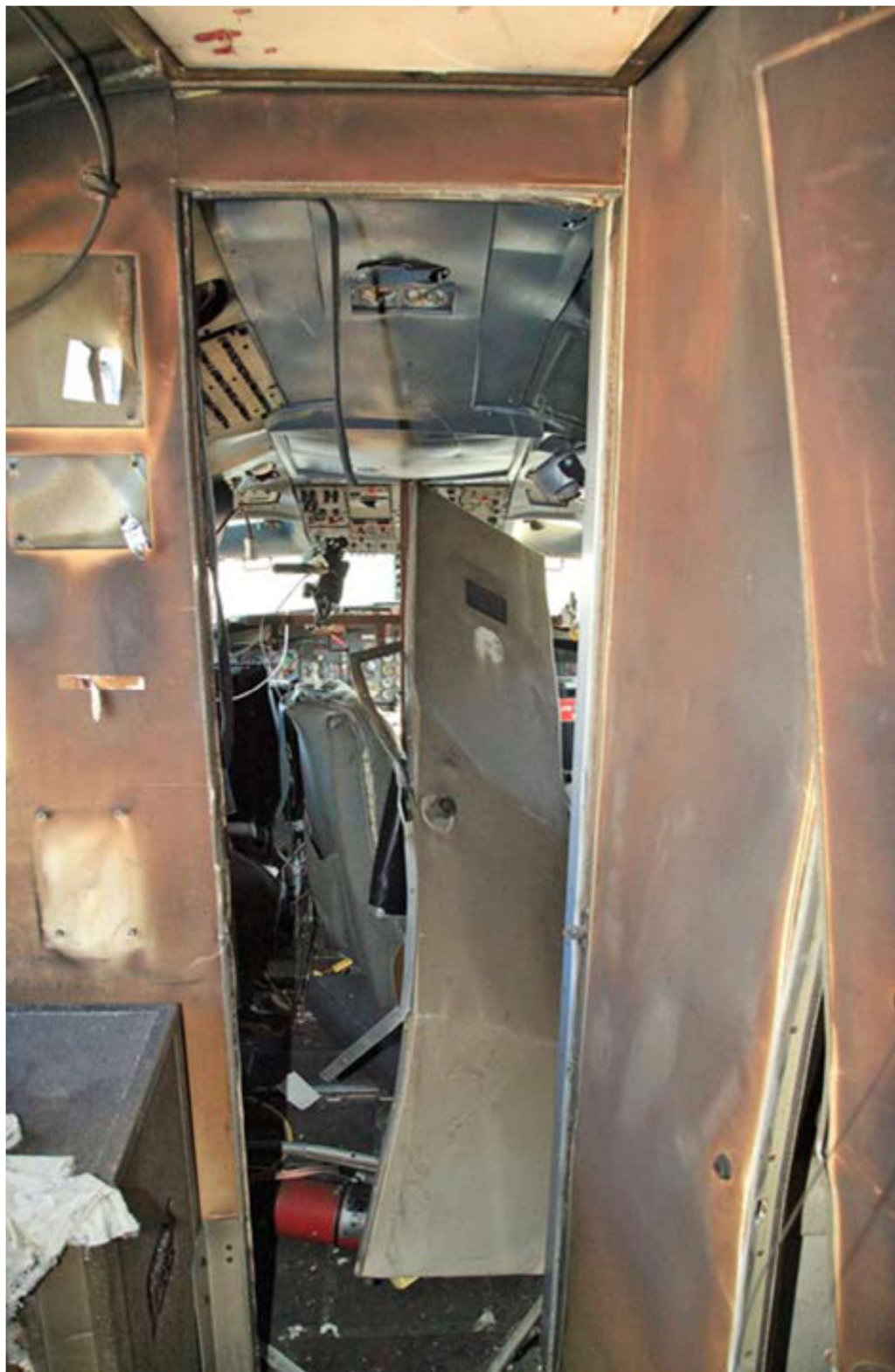
Figure 1.2: Aftermath of Explosion of Cargo Compartment from Lithium Battery Vent Gases
