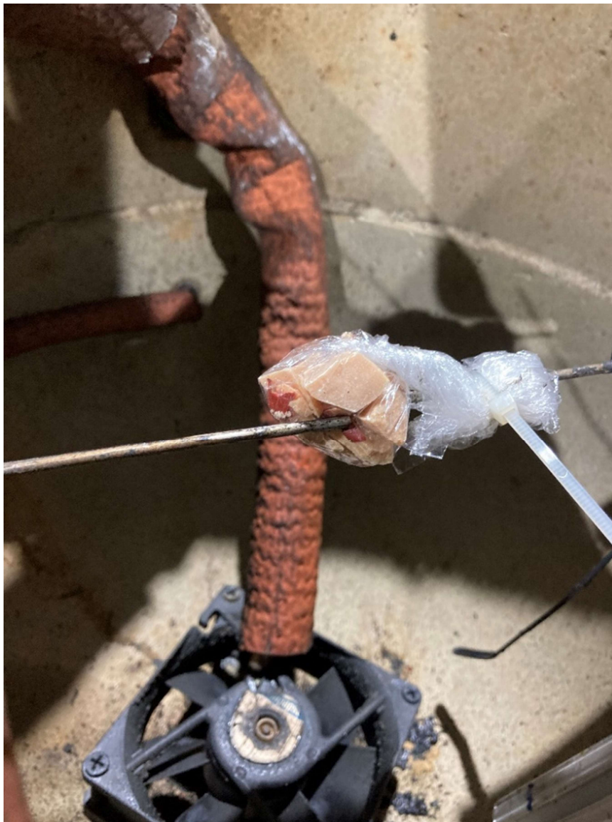
Figure 2.13: Final Method of Aerosol Activation. Aerosol was Sandwiched Within Cellophane Between the Igniter Probes.
