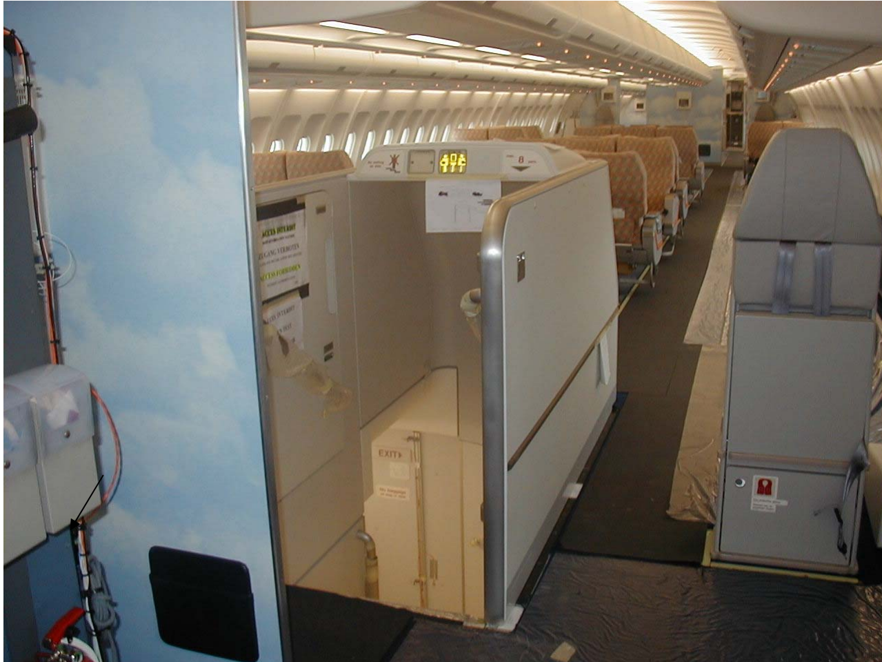
Staircase to lower deck facilities (Toilets & Stowage)
