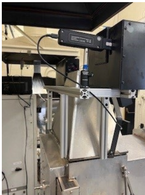
Figure 3: Platform and Power Meter (Protruding from Enclosure)
