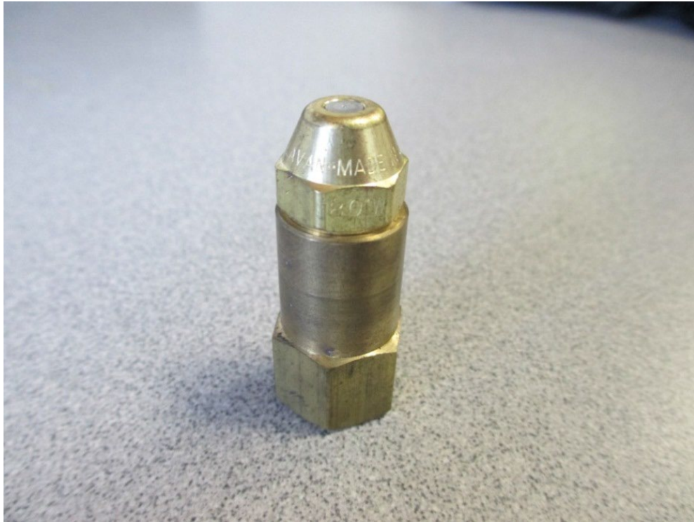
Figure K-18. Fuel nozzle and brass adapter
