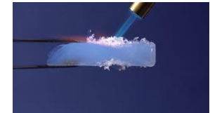
Mica materials for fire spread prevention prevent an ignited cell from affecting adjacent cells.
