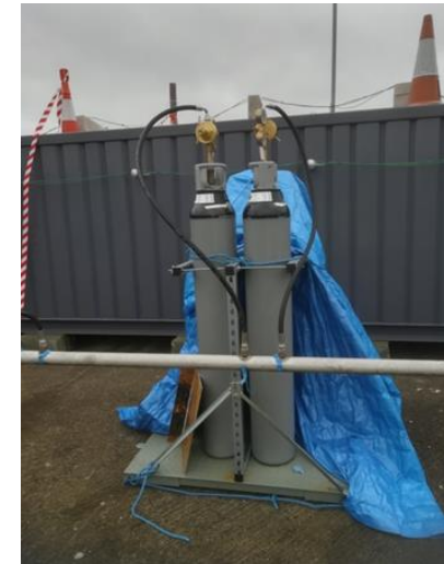
Nitrogen spray nozzle and nitrogen supply arrangement
