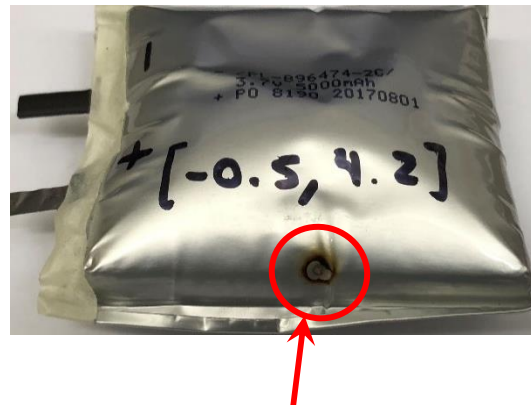
Burn from internal short circuit
