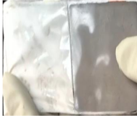
Fresh separator and anode during DPA
