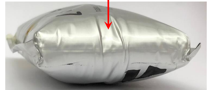
Swelling of damaged cell due to electrolyte decomposition
