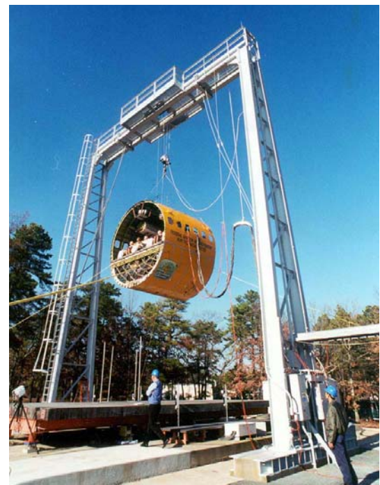
Figure 2. Dynamic Drop Test Facility
