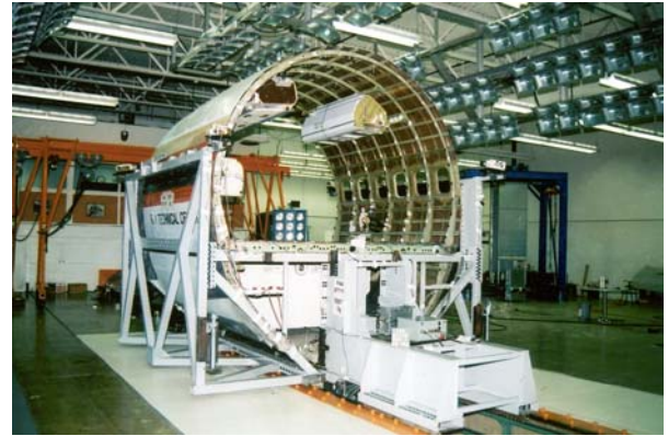
Figure 1. Longitudinal Impact Simulator Facility
