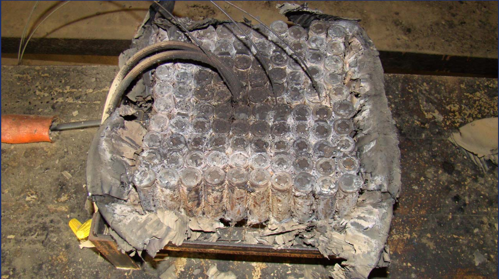
Bulk Load Configuration after Testing
