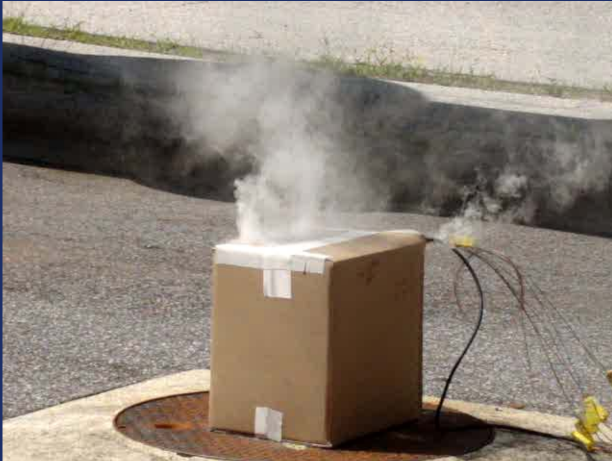
Oxygen Canister Container with Lithium Ion Cells
