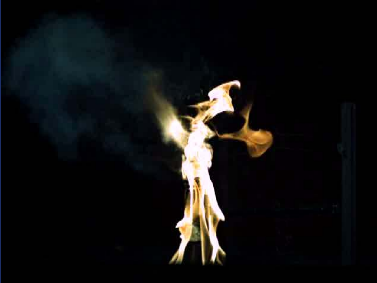
Lithium-Ion Cell in Thermal Runaway & Exploding
