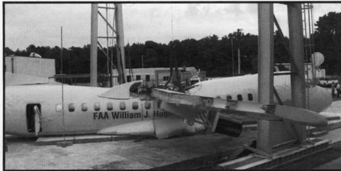
Figure 31 - Post Test View of Wing Penetration Into the Passenger Cabin
